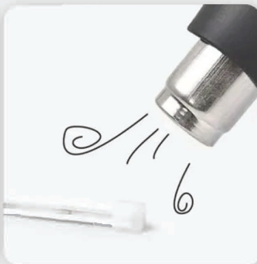
5. Blow dry the end cap with hot air to make the installation firm.
